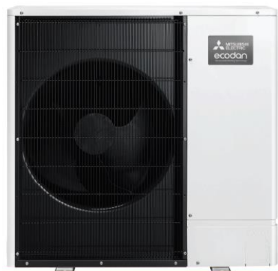
Figure A3: Example air source heat pump - Mitsubishi Ecodan 11.2kW PUHZ-W112VA (A++ rating, quiet at 45dbA at 1m, SCOP 3.5 @55C, SCOP 4.35 at 35C)
