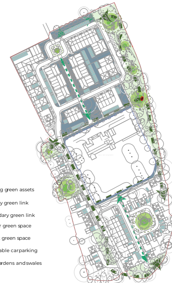
Figure 10. Proposed green and blue infrastructure, integrating SuDs with amenity and ecological enhancement.
